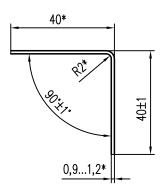
1. Материал сталь OU  $\frac{6-\Pi H \ \Gamma OCT \ 19904}{08 \ B\Gamma \ \Gamma OCT \ 14918}$ ; OU  $\frac{6-\Pi H \ \Gamma OCT \ 19904}{08 \ nc \ B\Gamma \ \Gamma OCT \ 14918}$ ; OU  $\frac{6-\Pi H \ \Gamma OCT \ 19904}{08 \ nc \ B\Gamma \ \Gamma OCT \ 14918}$
