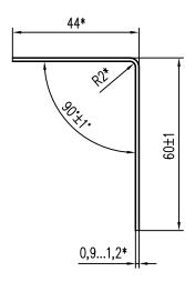
1. Материал сталь OU  $\frac{6-\Pi H \ \Gamma OCT \ 19904}{08 \ B\Gamma \ \Gamma OCT \ 14918}$ ; OU  $\frac{6-\Pi H \ \Gamma OCT \ 19904}{08 \ nc \ B\Gamma \ \Gamma OCT \ 14918}$ ; OU  $\frac{6-\Pi H \ \Gamma OCT \ 19904}{08 \ nc \ B\Gamma \ \Gamma OCT \ 14918}$
