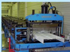
The lines can be equipped with flying scissors that provide a production capacity of 60 m/min, i.e. 20 sheets (4 min length) per minute.
