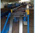
Roll-forming lines **LPSHR** series are designed for manufacturing "splint rail" type profile.
