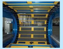
Bending machines of MGPL series are designed for bending sheet panels with a radius of 12 m to 100 m.
