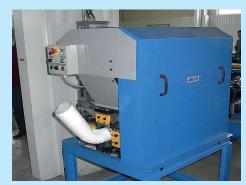
Bending Machines MGRP series are designed for manufacturing corrugated rectangular pipe bends with the required bending radius.
