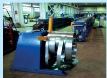
Roll-forming lines **LPP** series are designed for manufacturing panels of various configurations (racking systems, linear and other front panels).
