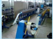
Roll-forming lines **LPKP** series are designed for manufacturing profiles for fixing front panels, facing of buildings, etc.
