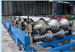
**LPRF (single purpose)** series are designed for manufacturing only one type of corrugated profile (corrugated board, cassette profile, panels of prefabricated buildings, etc.) with a width up to 1600 mm, thickness up to 3 mm, and profile depth up to 250 mm. The maximum profiling speed is 40 m/min.
