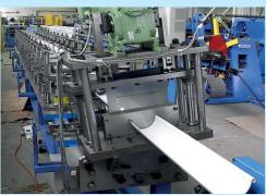
LPPT series are designed for LPZH series are designed for manufacturing rectangular cross section gutters of various dimensions.
