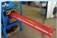
LPS series are designed for manufacturing siding-panels ("ship board", "L-beam", "log", "beacon", "angle", etc.), decorative profiles, profiles for fixing plasterboard plates, and other special profiles.
