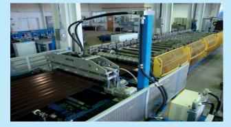
**Conveyors and stackers** are designed for stacking sheets in a pack and transferring them along and across the profiling axis.
