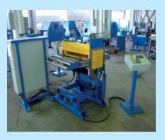
**Flying scissors** integrated in roll-forming lines are designed for cutting steel profiles to pieces without stopping.
