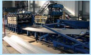
**Perforating machines** are designed for making spherical deformation plots on the original strip by means of rotation in order to increase its rigidity.
