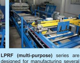
LPRF (multi-purpose) series are designed for manufacturing several types of corrugated profiles using one piece of equipment (profile depth from 8 mm up to 75mm). Tool change is carried out by use of quickly removable modules. Change-over time to move from one profile to another is 20 minutes. The lines can be equipped with flying scissors that provide a production capacity of 12 sheets (6 m in length) per minute.
