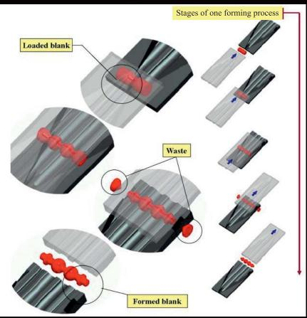
An exceptionally stable base together with extra-long dies give all cross-wedge rolling machine the capability of producing complex shapes and forms in one simple operation.
